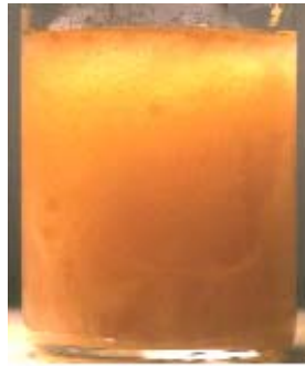
Glycol/Water solution at cloud point
