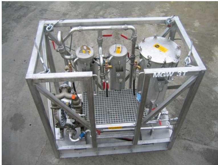
Filtration skid with pump
