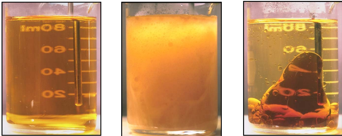
Figure 7 - 5 Temperature Sequence of Glycol Cloud Point Formation
